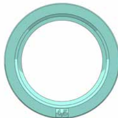
Marking for short lengths of pipe (4 m or 4.5 m) at the front of the socket.
